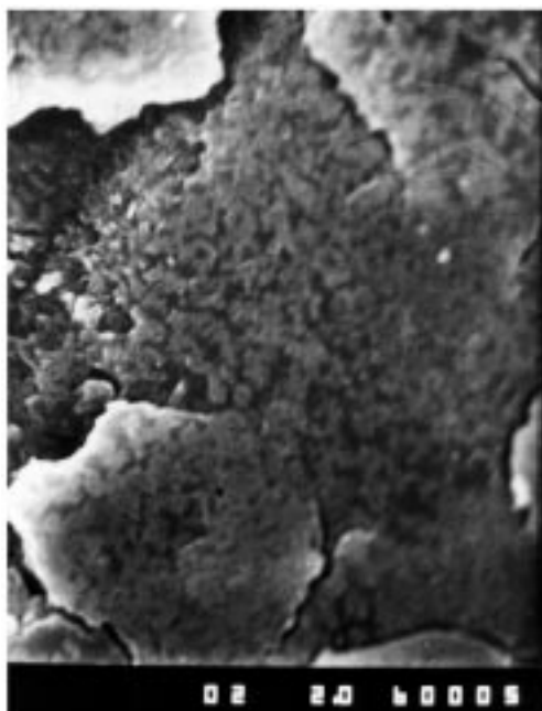
Figure 4. SEM micrograph of poly(N-methylaniline) (Magnification 800X)
