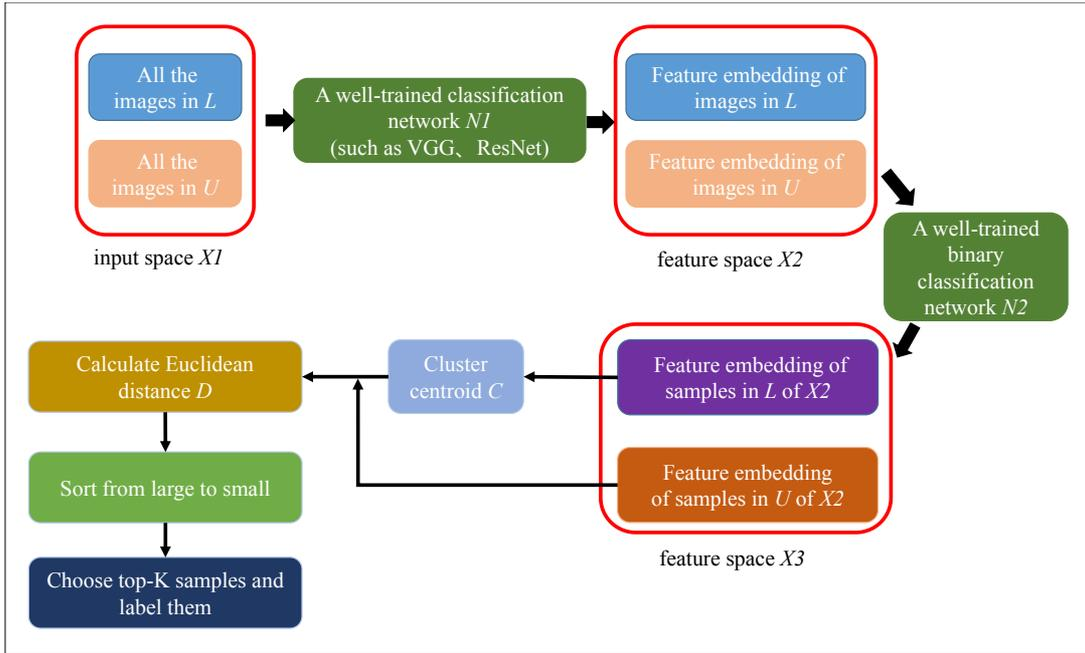
Figure 4. The proposed DBAL method.
