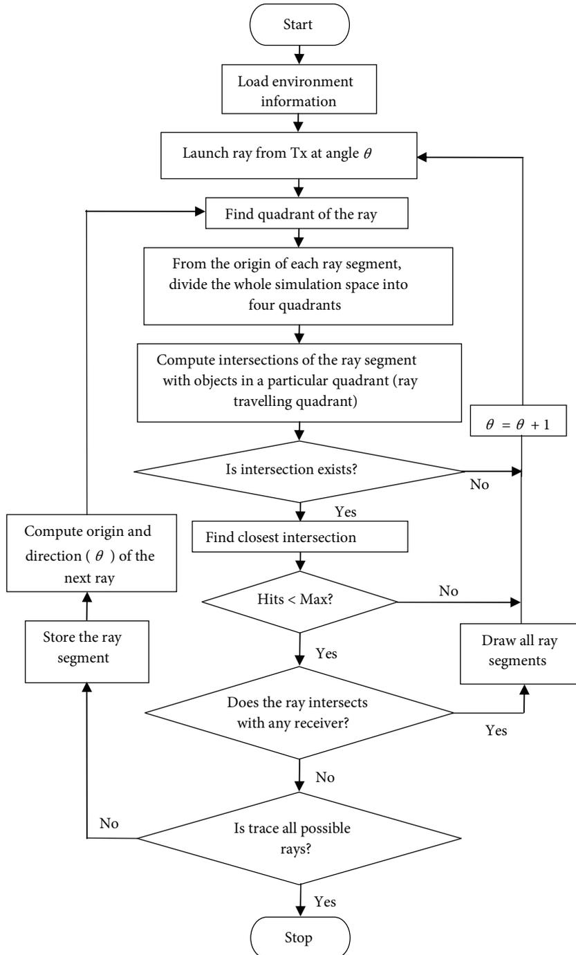
Figure 5. Simplified flowchart of the proposed algorithm.
