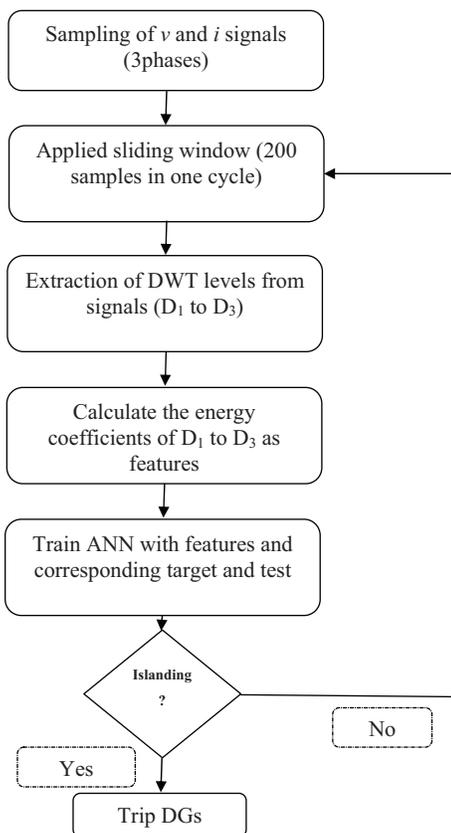
Figure 8. Flowchart of proposed algorithm.
