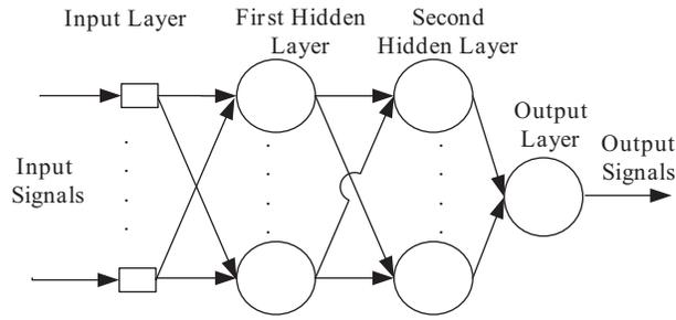
Figure 3. General structure of a neural network.
