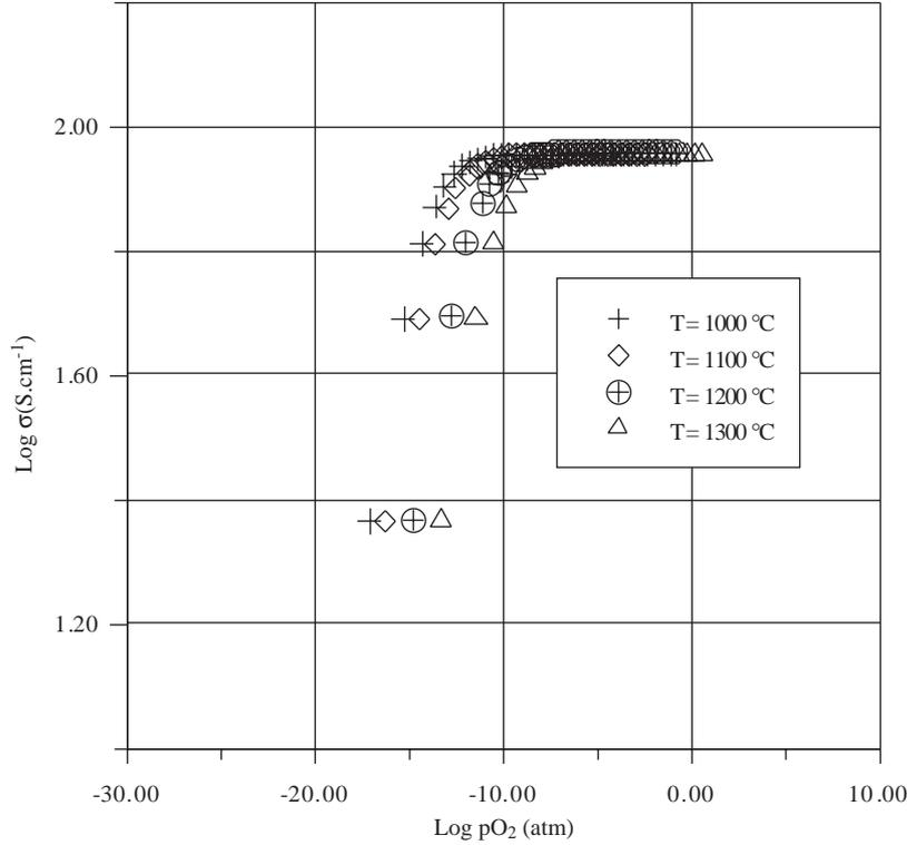
**Figure 7.** Electrical conductivity of La<sub>0.9</sub> Sr<sub>0.1</sub>Cr O<sub>3-δ</sub> as a function of pO<sub>2</sub> at 4 temperatures.
