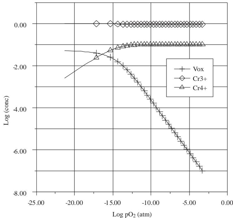
**Figure 1.** Defect diagram for LSC10 at 1000 °C.
