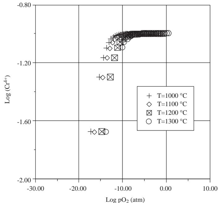
**Figure 2.** Relative carrier concentration as a function of pO<sub>2</sub> and temperature for LSC10.
