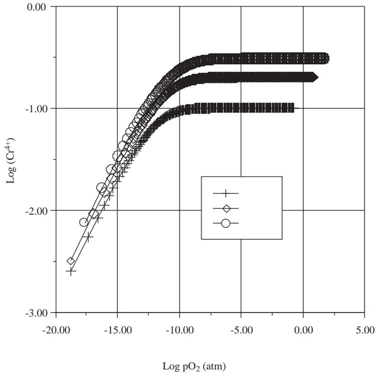
**Figure 3.** Relative carrier concentration as a function of pO<sub>2</sub> and composition at 1200 °C for LSC10.
