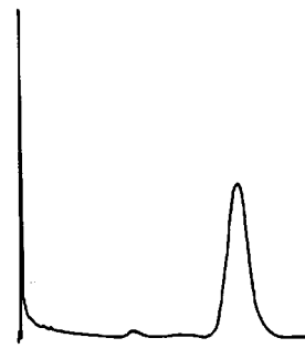
Figure 4. Chromatogram showing amount of standard DDT after the injection of 60 ng/ml to GLC.
