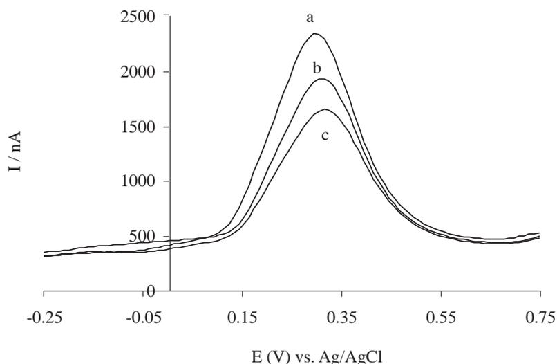
**Figure 2.** Square wave voltammograms of 0.1 mM NE in 0.1 M Tris-HCl buffer at pH 7.0 (a) without DNA (b) in the presence of 0.25 mM DNA and c) 2 mM DNA. Equilibrium time: 10 s, Frequency: 10 Hz, Step Potential: 5 mV, Amplitude: 25 mV.
