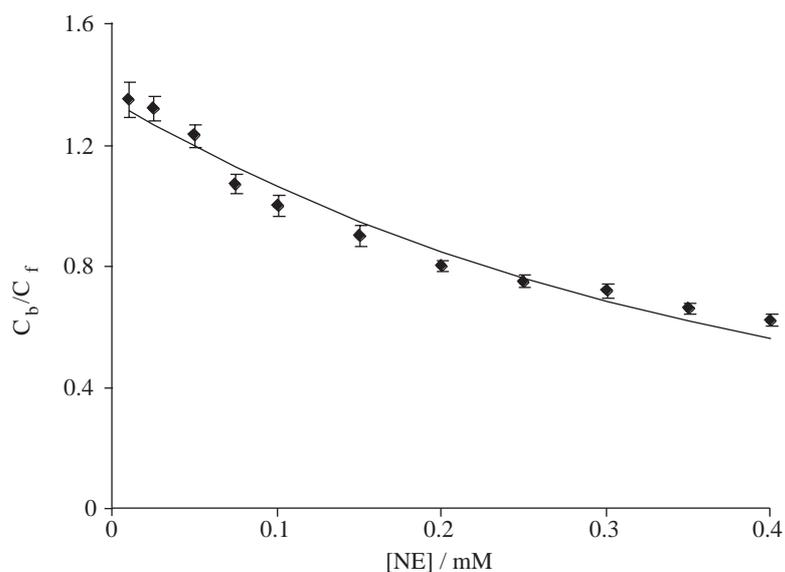
**Figure 4.** A plot of the ratio of  $C_b/C_f$  vs.  $C_T$  from the square wave voltammetric titration of NE against 2.0 mM DNA. The solid line shows a least squares fit to the data. Error bars were calculated at 95% confidence intervals from 5 different runs.
