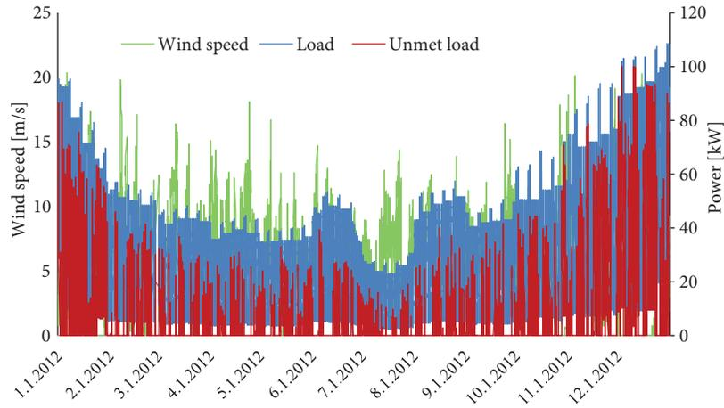
**Figure 7.** Load profile [kW] and unmet load [kW] vs. wind speed [m/s] during the year for hybrid power system configuration in Case II.
