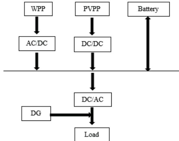
Figure 3. Diagram of the proposed hybrid power system.
