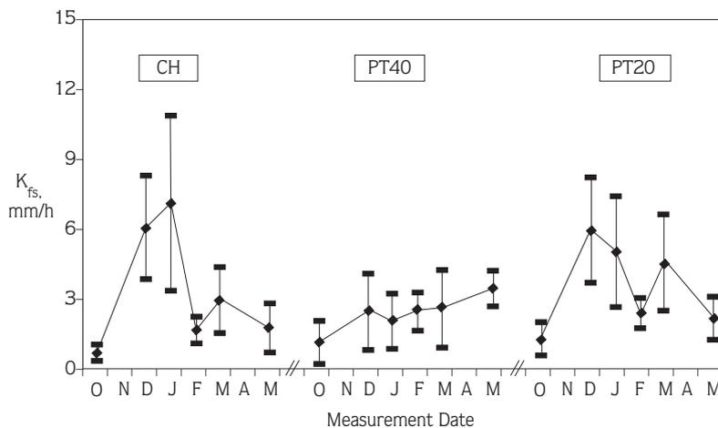
Figure 2. Mean  $K_{fs}$  values of the plots with their standard deviations for each measurement date and tillage system.
