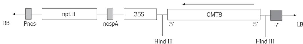
Figure 1. Schematic representation of the T-DNA region of the *pOMT8* antisense construct in the binary vector pGA643. 35S, 35S RNA promoter of cauliflower mosaic virus; nosP, promoter of the nopaline synthase gene; nospA, terminator of the nos gene. RB, LB are the right and left borders of the T-DNA.
