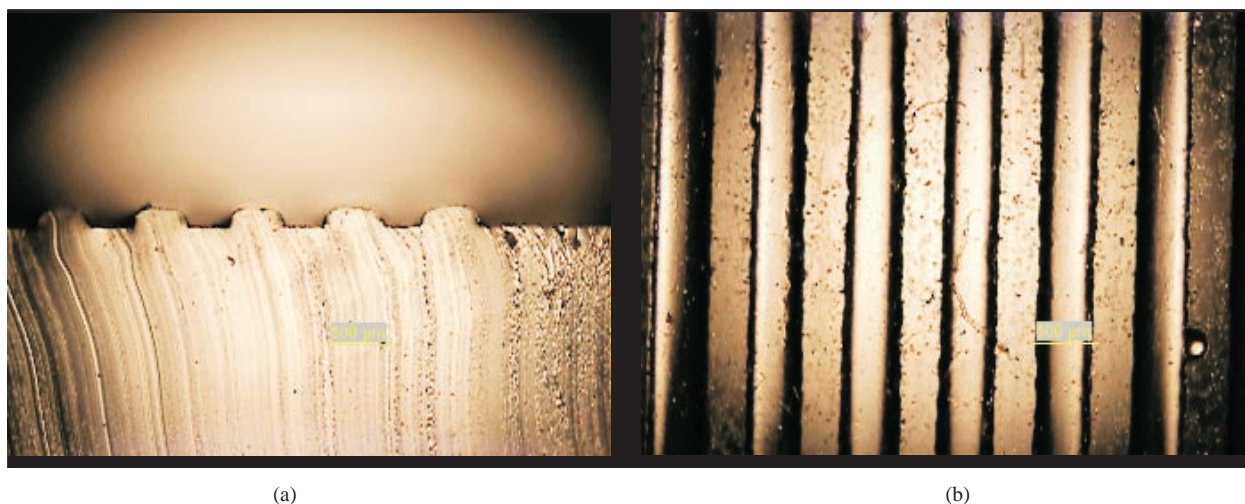
Figure 1. Optical microscopic images of the PDMS stamps. The bar represents 300 \mu\text{m} . (a) cross-sectional view, (b) front view.
