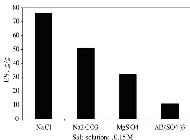
**Figure 11.** Swelling capacity of the hydrogel as a function of ionic strength of the salt solution. Reaction conditions: collagen 3.0 g, MBA 0.008 mol/L, AMPS 0.68 mol/L, APS 0.015 mol/L, 80 °C, 60 min.
