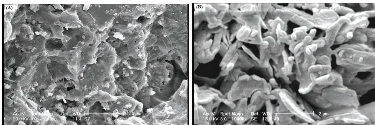
**Figure 2.** SEM photograph of the optimized superabsorbent hydrogel (collagen 3.0 g, MBA 0.008 mol/L, AMPS 0.68 mol/L, APS 0.015 mol/L, 80 °C, 60 min). (A) Surface of porous hydrogel; (B) Cross-sectional area of porous hydrogel. The average pore diameter of the synthesized hydrogel was 16.7 nm.
