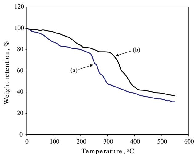
**Figure 3.** TGA of collagen (a) and collagen-g-poly(AMPS) hydrogel (b).
