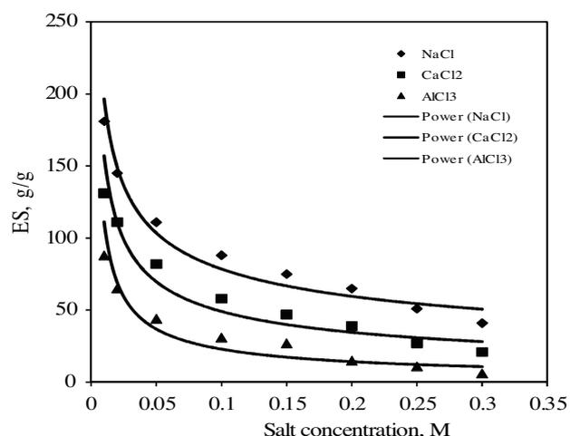
**Figure 10.** Swelling capacity variation of the hydrogel in saline solutions with various concentrations. Reaction conditions: collagen 3.0 g, MBA 0.008 mol/L, AMPS 0.68 mol/L, APS 0.015 mol/L, 80 °C, 60 min.
