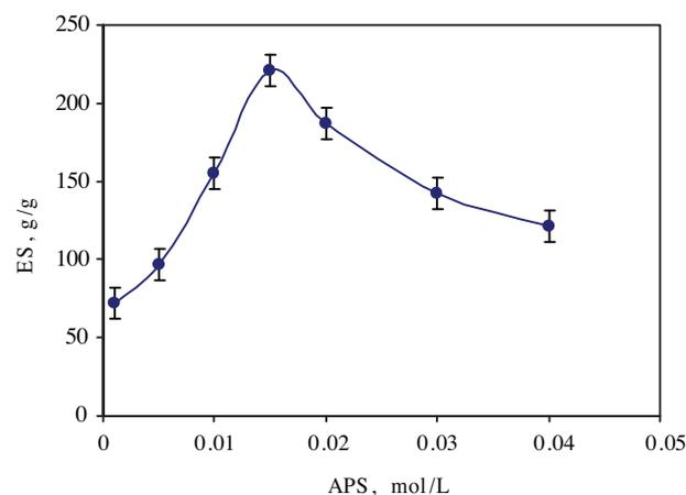
**Figure 6.** Effect of initiator concentration on swelling capacity. Reaction conditions: collagen 2.0 g, MBA 0.008 mol/L, AMPS 0.68 mol/L, 80 °C, 60 min.
