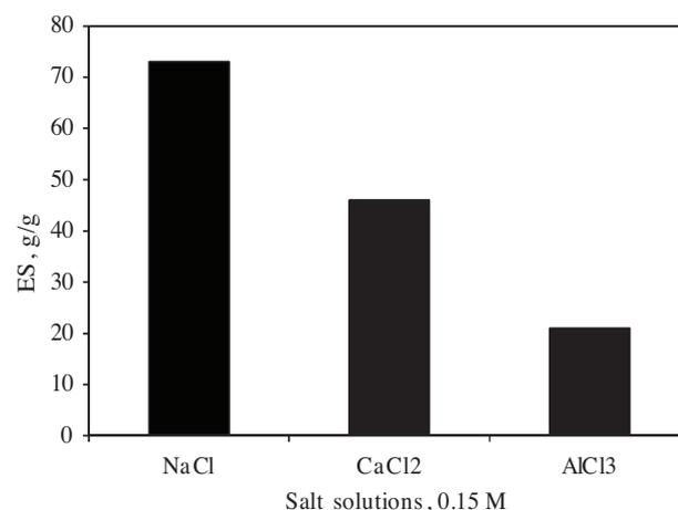
**Figure 8.** Swelling capacity of the hydrogel in different chloride salt solutions (0.15 M). Reaction conditions: collagen 3.0 g, MBA 0.008 mol/L, AMPS 0.68 mol/L, APS 0.015 mol/L, 80 °C, 60 min.
