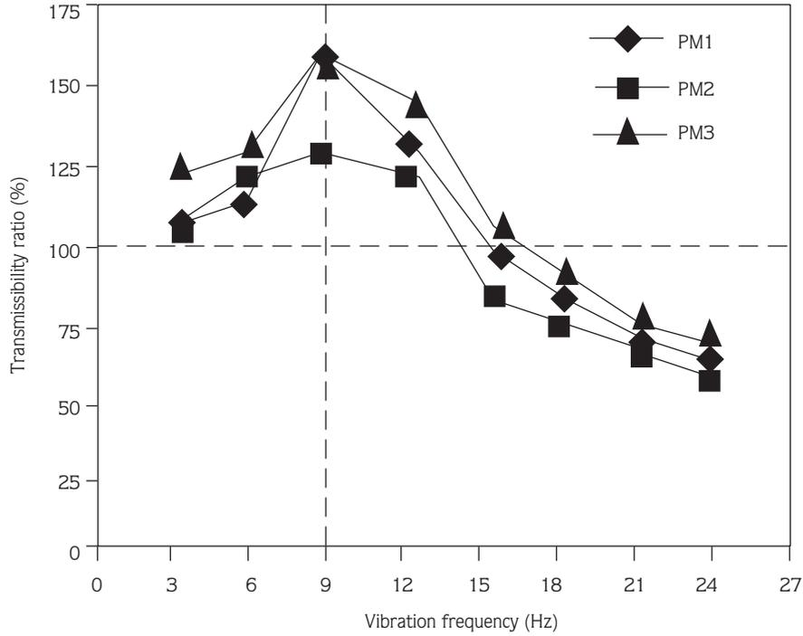
Figure 5. Transmissibility ratio of 3 packaging methods.
