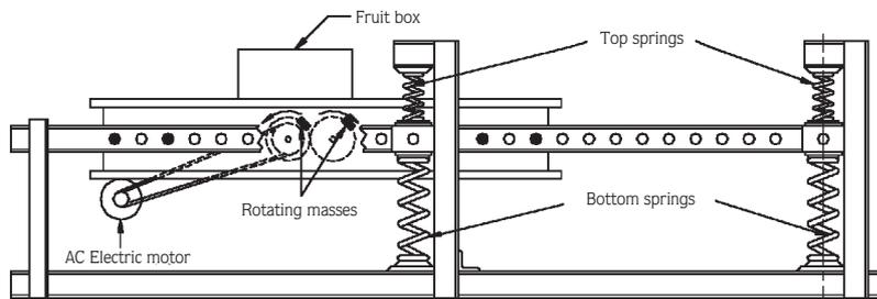
Figure 1. Laboratory vibration simulator.
