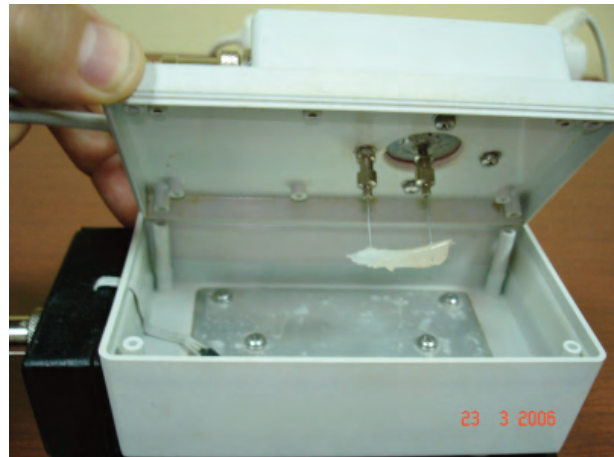
Figure 2. Fish muscle sample placed on needle electrodes of the measuring box.
