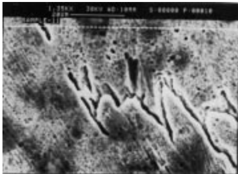
Figure 5. Scanning electron micrographs of hot cracks in welded zone.
