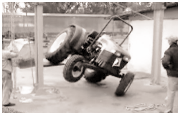
Figure 3. Determining the lateral stability of a tractor on the reclining platform.
