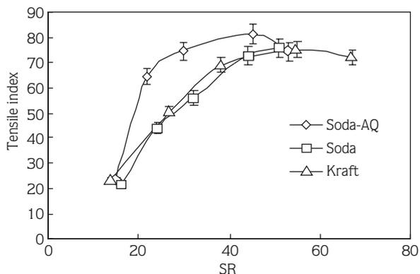
Figure 3. Relationship between SR value vs tensile of *Acacia auriculiformis* pulp from kraft, soda and soda-AQ process.
