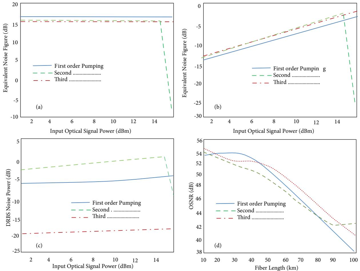
**Figure 3.** First, second, and third order pumping configurations plots for (a) equivalent noise figure (dB), (b) OSNR (dB), (c) DRBS noise power (dB) vs. input optical signal power (dBm), and (d) OSNR (dB) vs. fiber length (km).
