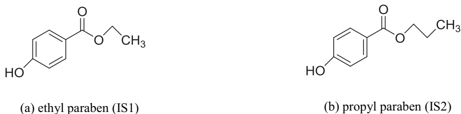
Figure 2. Chemical structures of (a) ethyl paraben (IS1) and (b) propyl paraben (IS2).
