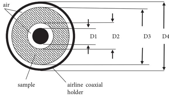
**Figure 3.** The sample in a coaxial sample holder with an air gap.
