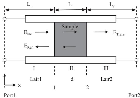
**Figure 2.** Transmitting of electromagnetic waves through and reflecting from a sample in a transmission line [26].
