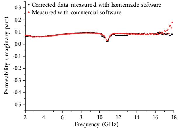
**Figure 7.** Comparison of results obtained with commercial and our own software for the imaginary part of the permeability of the sample.
