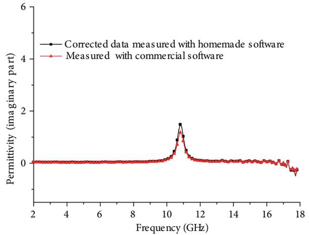
**Figure 5.** Comparison of results obtained with commercial and our own software for the imaginary part of the permittivity of the sample.
