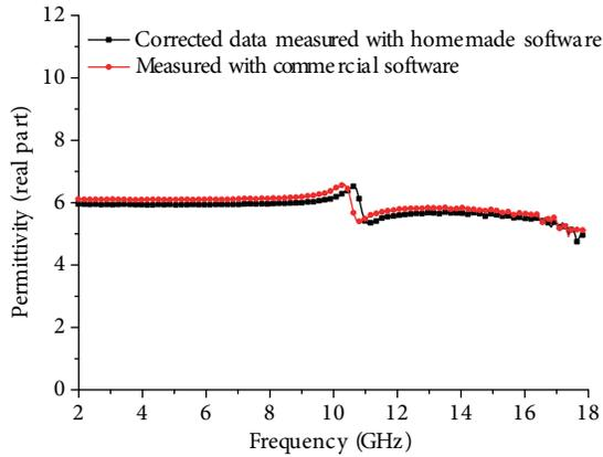
**Figure 4.** Comparison of results obtained with commercial and our own software for the real part of the permittivity of the sample.
