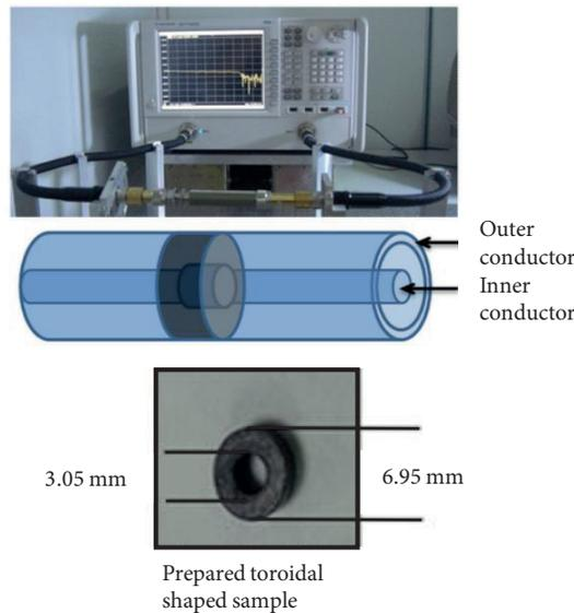
**Figure 1.** The S parameter measurement test setup for using a two-port VNA (top), a schematic representation of sample inside the sample holder (middle), and picture of prepared sample (bottom).
