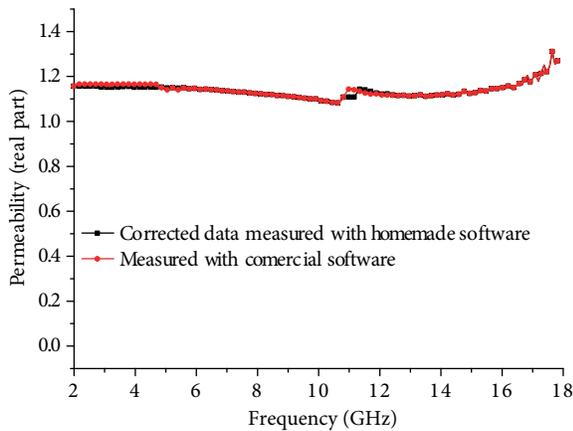
**Figure 6.** Comparison of results obtained with commercial and our own software for the real part of the permeability of the sample.
