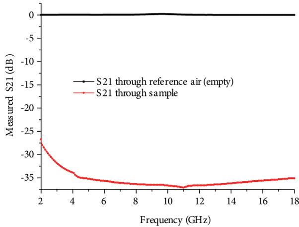
**Figure 8.** Insertion loss measurement in terms of S21 parameters.
