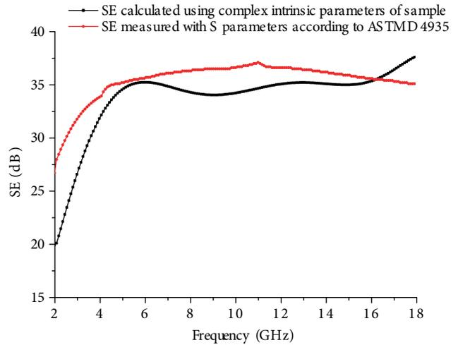
**Figure 11.** SE measurement according to the definition of SE given in ASTM ES7-83 Standard and SE calculated using intrinsic parameters of the sample with the NRW method.
