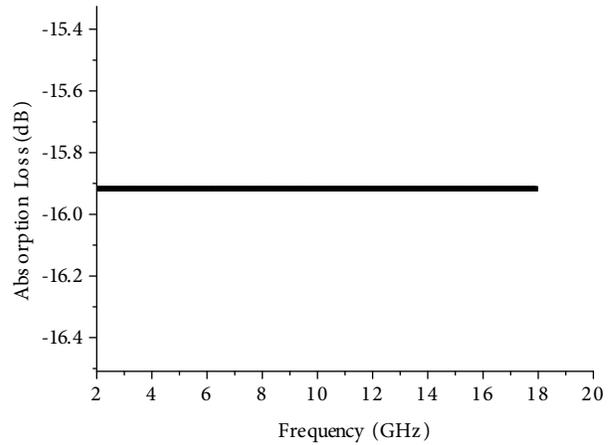
**Figure 9.** Frequency dependence of the mean value of the absorption loss.
