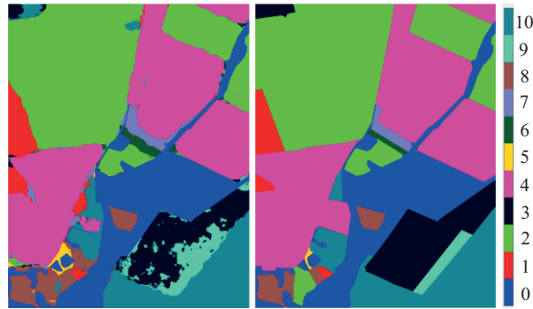
Figure 5. (Left) One of the results of the proposed method (dimension = 9, training sample size for each class = 100, accuracy = 0.8989, kappa = 0.8643); (Right) Ground-truth.
