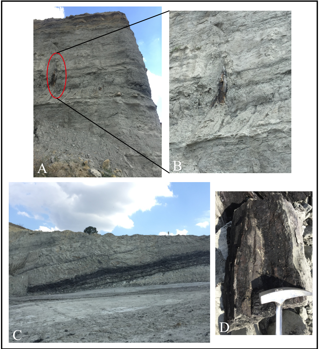
Figure 3. A,B) The view of the horizontal or nearly horizontal layers of the Danişmen Formation in the Keşan region and tree trunks perpendicular to these layers. C) The view of the layers forming the formation and the coal layer in the coal mine. D) View of the carbonated tree trunks extracted from near the coal layer.
