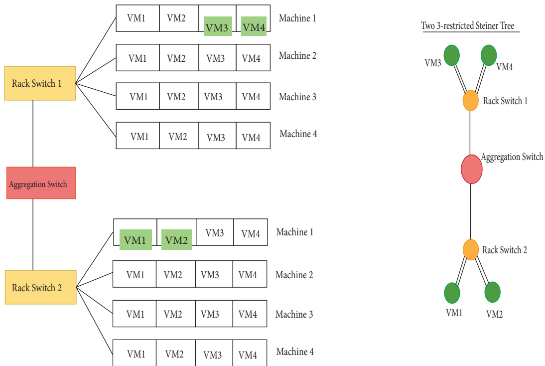
Figure 2. Steiner tree for VDC distribution.
