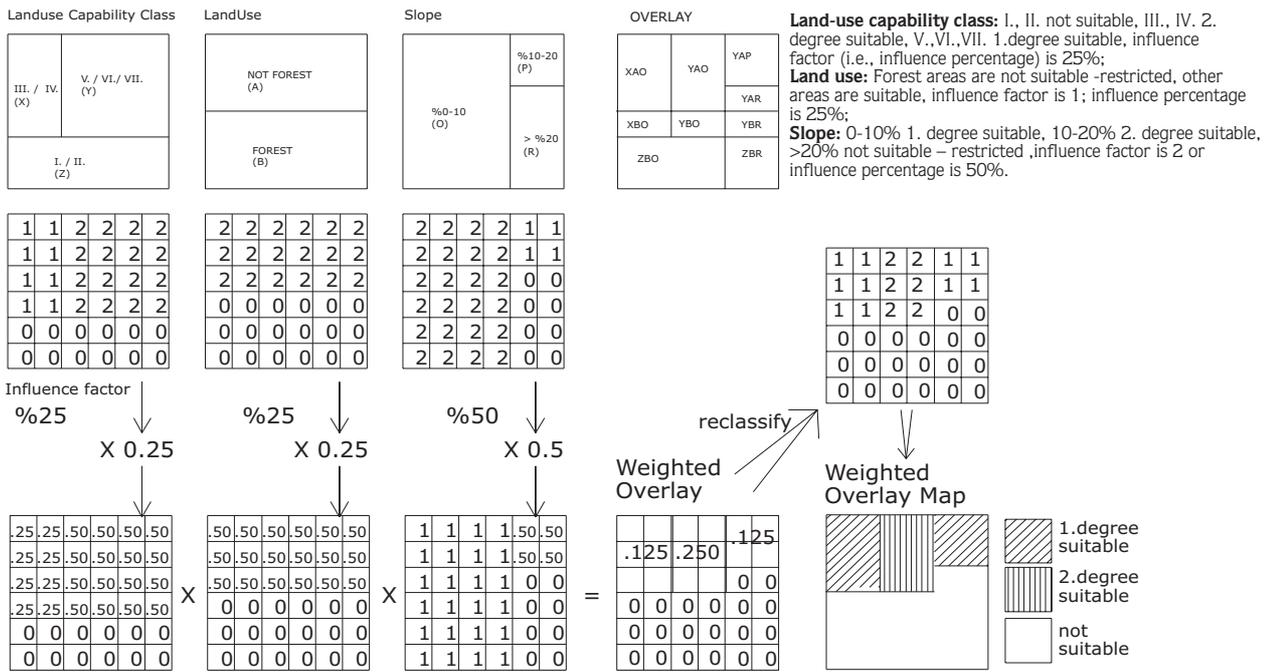
Figure 3. A hypothetical example for the weighted overlay method (from Çabuk 2001).
