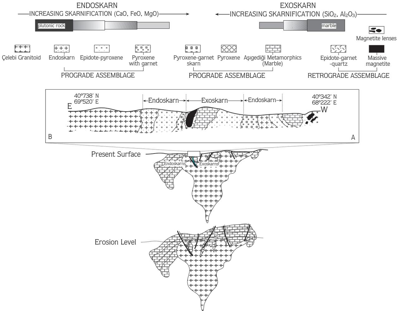
**Figure 3.** A schematic diagram illustrating the skarn zones. Prograde and retrograde assemblages and relative setting of skarn zones in the Çelebi district.
