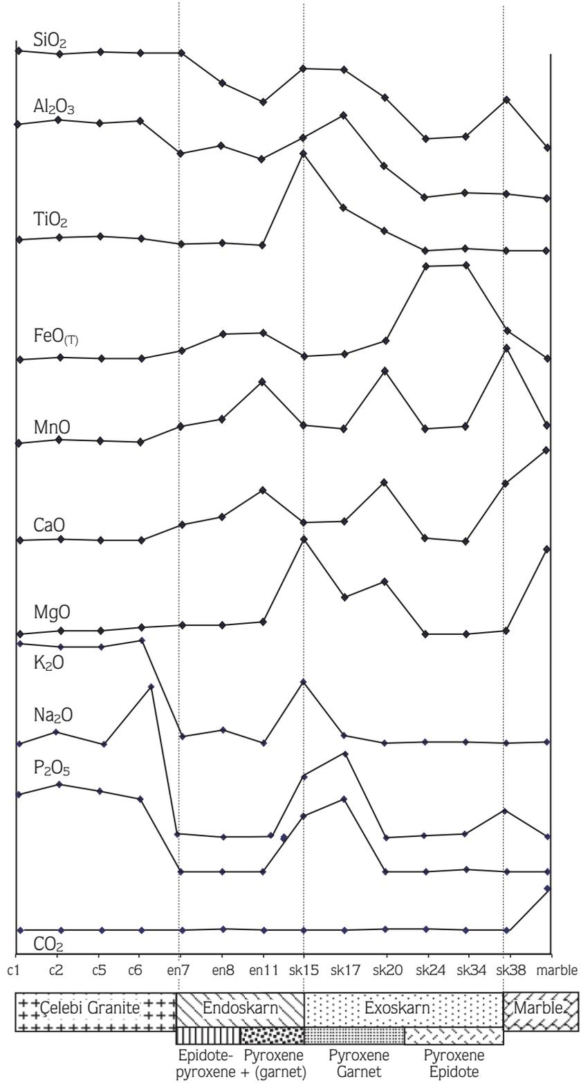
Figure 4. The profiles from granitoid to marble showing the distribution and abundance of elements in skarn zones.
