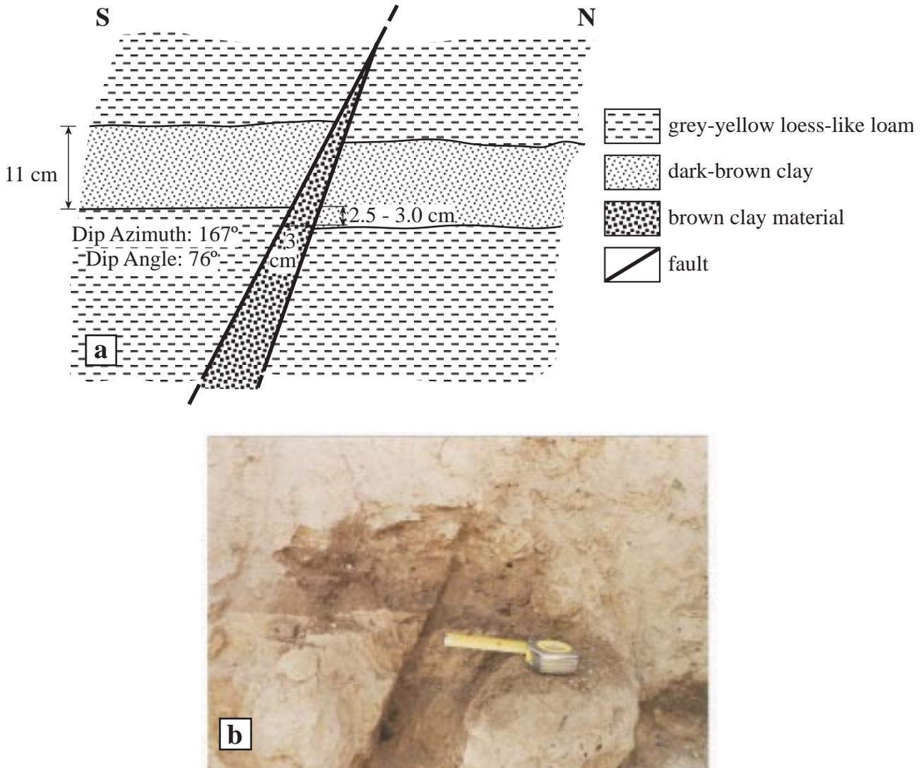
Figure 17. Field sketch (a) and photograph (b) of a seismic fracture in the western wall of the Talgar fortress.
