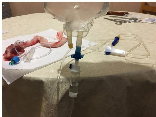
**Figure 2.** Measuring urethral closure pressure at different volumes of TCD's balloon.
