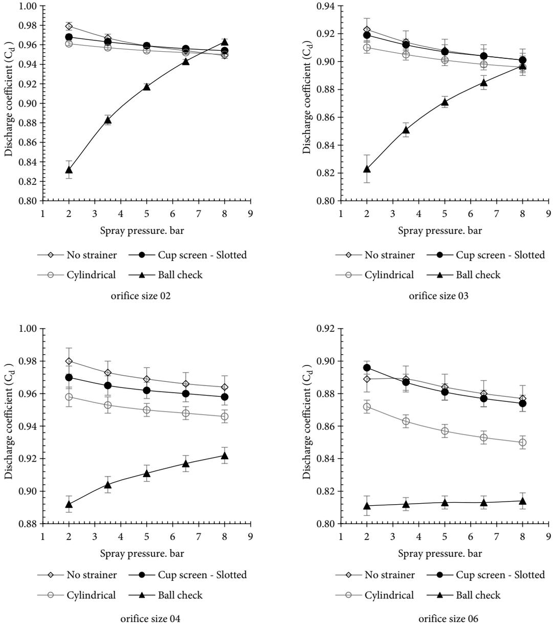
**Figure 2.** The influence of the strainer types on the variation of discharge coefficient ( $C_d$ , mean and standard error) corresponding to the different spray pressures for each of the nozzle orifice sizes.
