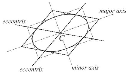
**Figure 13.** Axes and eccentricities of an ellipse.
