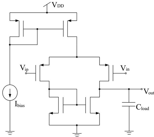
Figure 4. The schematic of the single stage amplifier.
