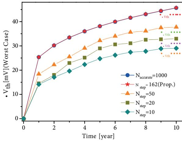
Figure 7.  $V_{th}$  degradation for different step counts.
