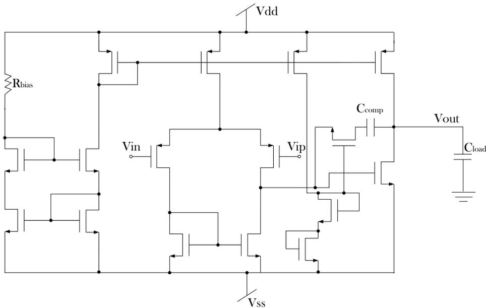
Figure 10. The schematic of a basic 2 stage OTA.
