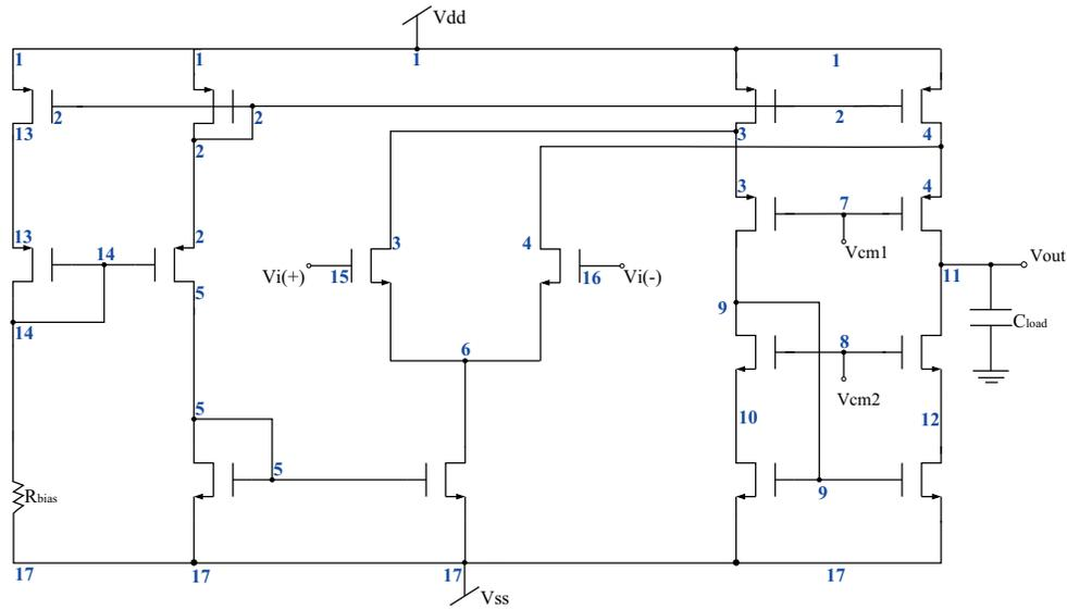
Figure 6. Schematic of the folded cascode amplifier.
