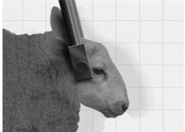
**Figure 3.** Electrode position for sheep (side view).
