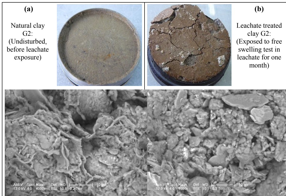
Figure 5. Snapshot and ESEM image of clay G2: a) before leachate, b) following the leachate exposure for 1 month (magnification is 4000 \times ).
