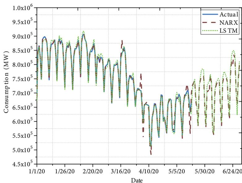
**Figure 12.** Six-month forecasting data and four-month real consumption data with NARX and LSTM.
