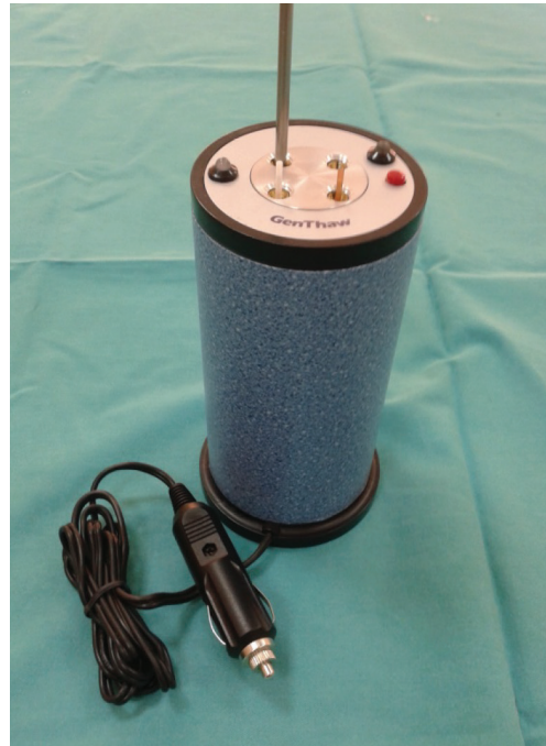
Figure. Dry thawing system working with 12–13.6 V, at adjusted temperature of 37 °C, with holes for 0.25 and 0.50 mL straws and for catheter.
