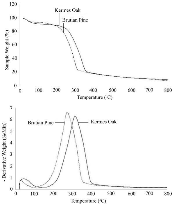
**Figure 3.** TGA (a) and DTG (b) thermograms of kermes oak and brutian pine fibers.
