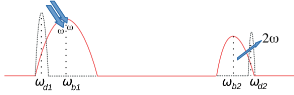
Figure 1. Illustration of the plasmonic dark modes coupled to the bright modes. Two \omega plasmons combine to generate 2\omega plasmons. Two distinct structures having dark resonances at \omega_{d1} and \omega_{d2} interacts with the FH ( \omega_{b1} ) and SH ( \omega_{b2} ) mode of the nonlinear structure, respectively.
