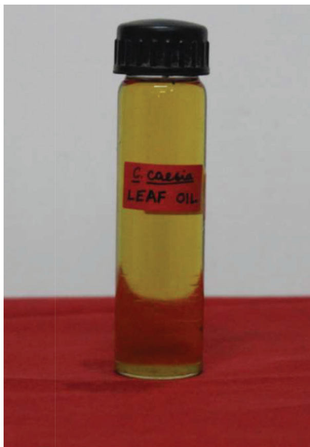
Figure 2. Essential oil extracted from the leaves of C. caesia through hydro-distillation at CSIR-NEST, Assam (India).
