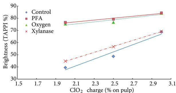
Figure 2. Effect of ClO<sub>2</sub> charge on the final brightness of bamboo pulp.
