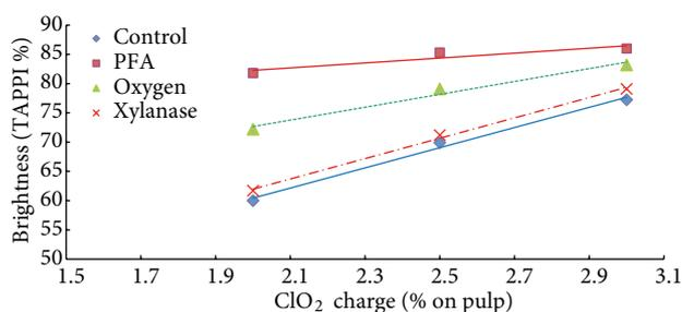
Figure 1. Effect of ClO<sub>2</sub> charge on the final brightness of hardwood pulp.
