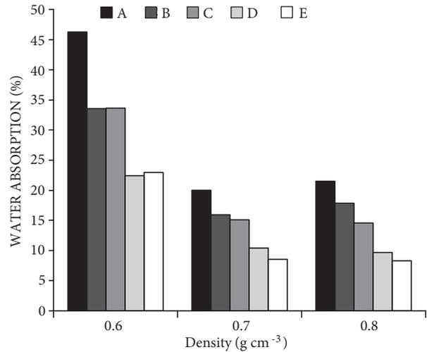
Figure 3. The 2-h water absorption of the panels.
