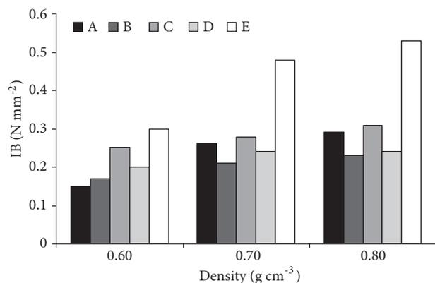
Figure 7. Internal bond strength of panels.
