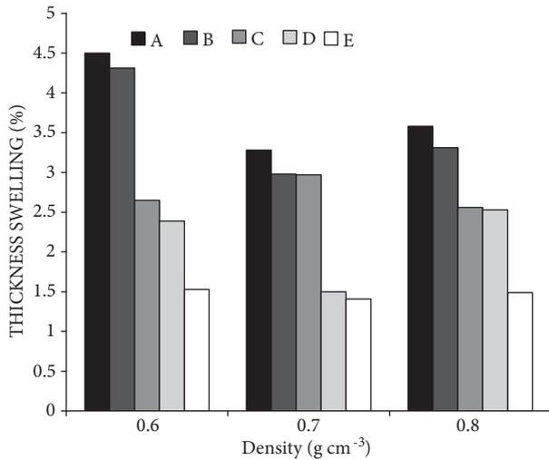
Figure 1. The 2-h thickness swelling of the panels.
