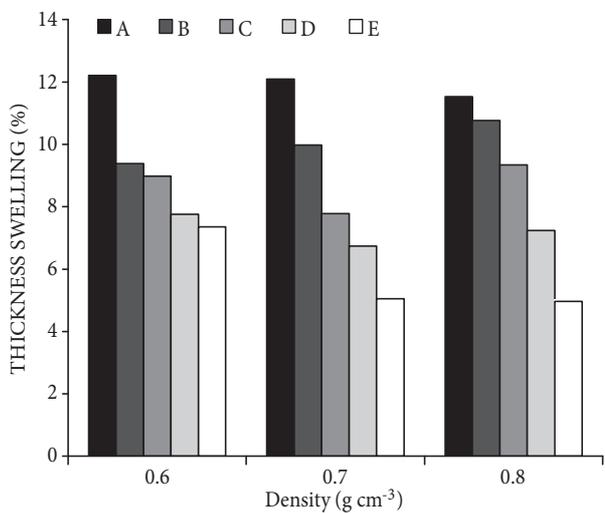
Figure 2. The 24-h thickness swelling of the panels.
