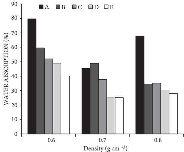
Figure 4. The 24-h water absorption of the panels.
