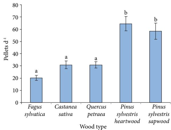
Figure 4. Effect of wood type on the feeding rate of *Limnoria quadripunctata*, as measured by faecal pellet production. Wood types with significantly different pellet production rates are indicated by different letters (GLM ANOVA with wood type as a fixed factor and pellets d<sup>-1</sup> square root transformed, Tukey's post hoc test)
