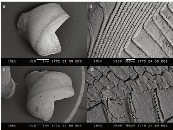
Figure 3. Air-dried shells of teredinids from the panels exposed at Mersin. a. Whole shell valve from *Pinus* heartwood. b. Detail of denticulated ridges of the anterior slope of the shell in Figure 3a. c. Whole shell valve from *Castanea*. d. Detail of Figure 3c showing older denticulated ridges obscured by the coating that was probably left by the *Castanea* heartwood
