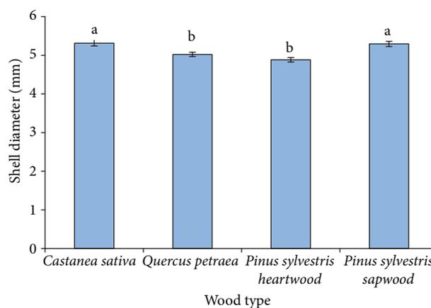
Figure 1. Diameter (mean  $\pm$  SE) of the shells of teredinid wood borers in panels of a range of commercial Turkish wood types exposed at Mersin, southern Turkey. Wood types with significantly different shell diameters are indicated by different letters (GLM ANOVA with wood type as a fixed factor and diameter log transformed, Tukey's post hoc test)
