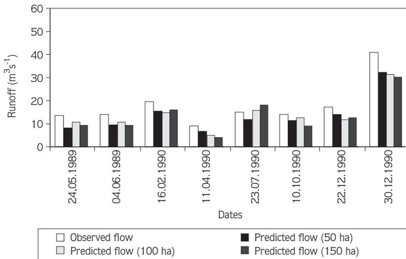
Figure 2. Comparison of predicted and observed average runoff rates at the outlet of the Rock Creek watershed using AGNPS.
