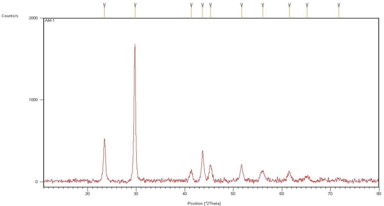
**Figure 1.** XRD pattern of Se-NPs.
