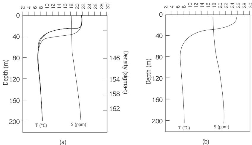
Figure 2. The salinity and temperature profiles are plotted against depth and water density in (a) October 1996, (b) July 1997. Measurements were repeated several times during the stay at the station 41°30' N, 39°45' E. The solid horizontal lines show the sampling layers.
