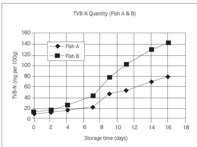
Figure 6. Comparison of TVB content in trout wrapped in aluminium foil (B) and in cling film (A) stored at 4-6°C (semi micro steam distillation method).
