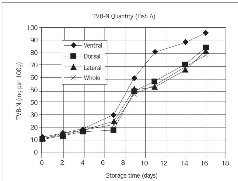
Figure 4. Concentration of TVB-N (mg N/100g) in various parts of fish wrapped in cling film stored at 4-6°C (semi micro steam distillation method).
