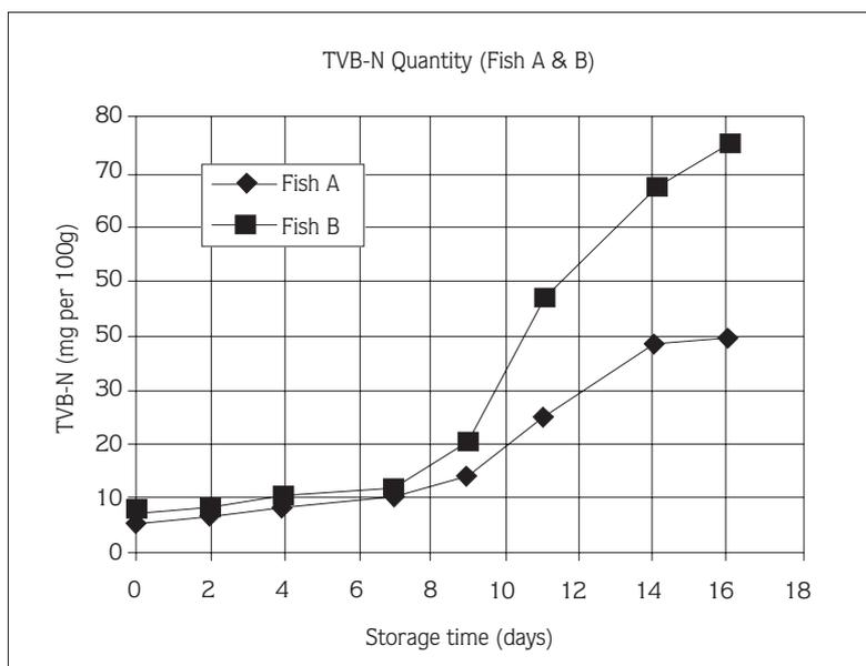
Figure 3. Comparison of TVB-N values in fish wrapped in aluminium foil (B) and in cling film (A) stored at 4-6°C (Conway micro-diffusion method).
