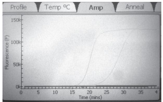
**Figure 2.** The display of the portable real-time instrument for LAMP reaction run and fluorescence detection.
