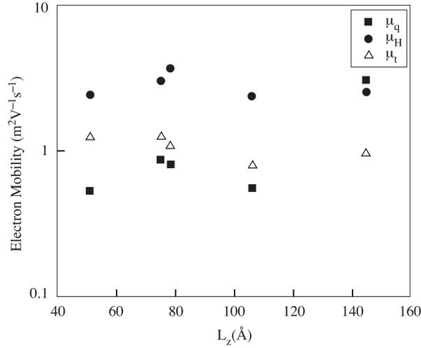
**Figure 8.** Low temperature electron mobilities versus quantum well width of the samples studied.
