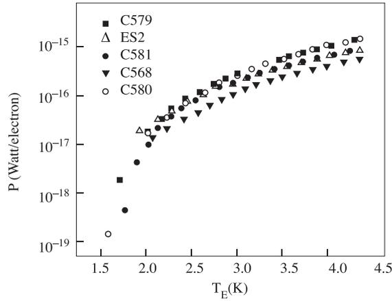
**Figure 6.** The power loss per electron versus electron temperature for all the samples studied [7].
