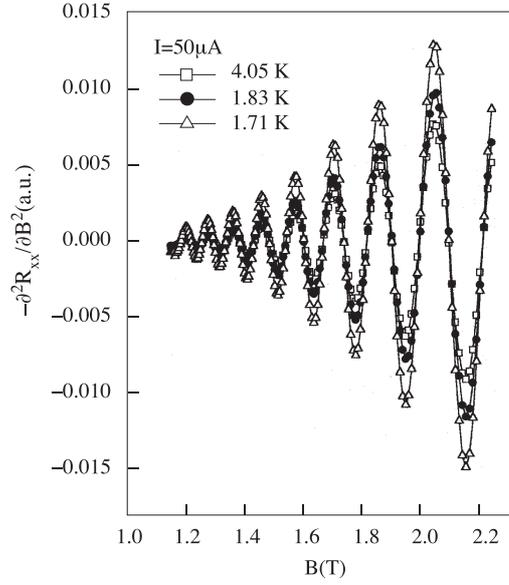
**Figure 4.** Experimental recordings of the SdH oscillations as a function of lattice temperature in sample C579.
