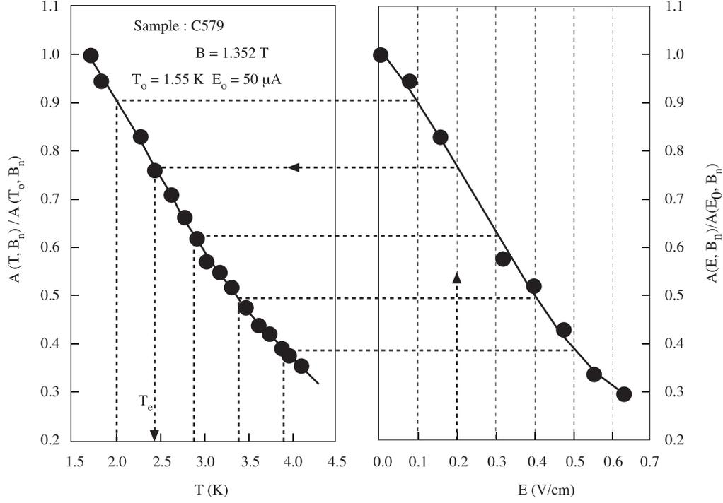
**Figure 5.** The electron temperature is obtained by comparing the lattice temperature and electric field dependencies of the amplitude of SdH oscillations.
