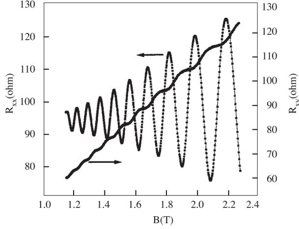
**Figure 1.** Magnetoresistance ( $R_{xx}$ ) and Hall resistance ( $R_{xy}$ ) as a function of magnetic field for sample C580 measured at 4.2 K [19].
