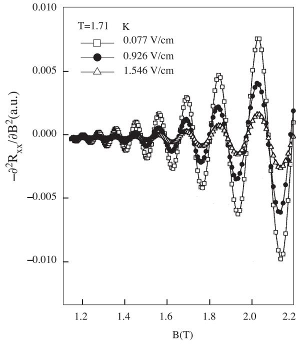
**Figure 3.** Experimental recordings of the SdH oscillations as a function of the applied electric field in sample C579.
