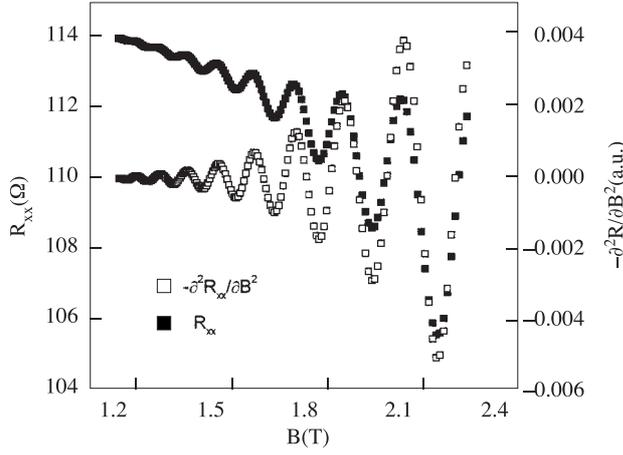
**Figure 2.** Magnetoresistance and its negative second derivative measured at 4.2 K in sample C579.
