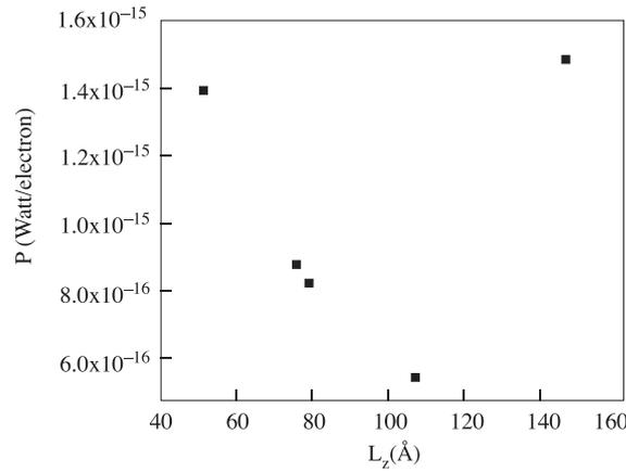
**Figure 7.** Quantum well - width dependence of power loss per electron at electron temperature 4.2 K.
