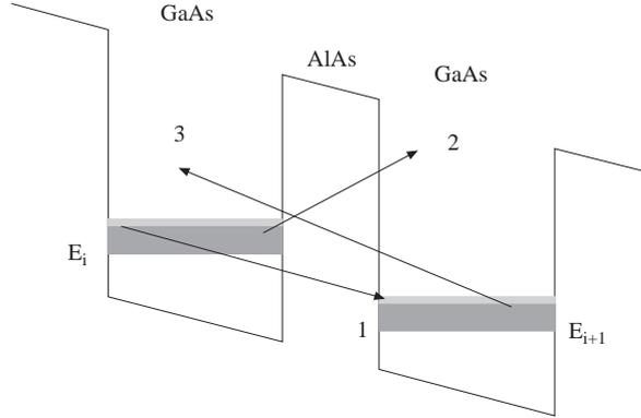
**Figure 1.** Possible phonon-assisted tunnelling transitions in a SL showing both stimulated phonon emission (1) and absorption (2,3) of phonons. For phonons with  $\mathbf{q}$  perpendicular to the plane of SL and for  $\hbar\omega = E_i - E_{i+1}$ , only transition (1) is allowed.
