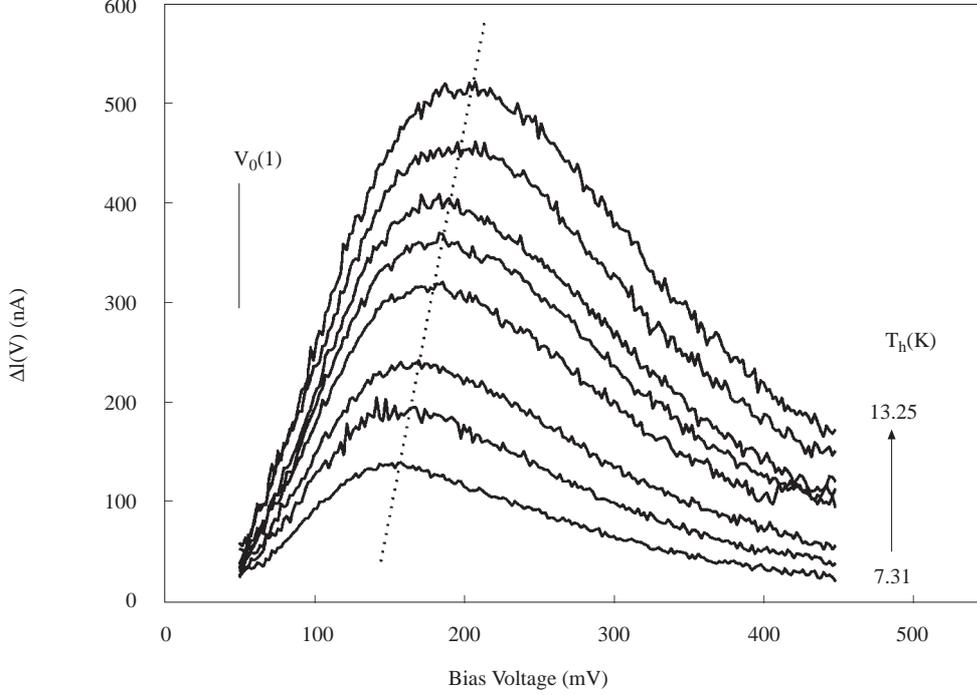
**Figure 3.** Dependence of phonon (TA) induced signal on bias voltage for different heater temperatures,  $T_h$ . This was obtained by measuring the signal at the maximum in  $\Delta I(t)$ . The dashed line shows the shift of the maximum in  $\Delta I(V)$  with  $T_h$ .
