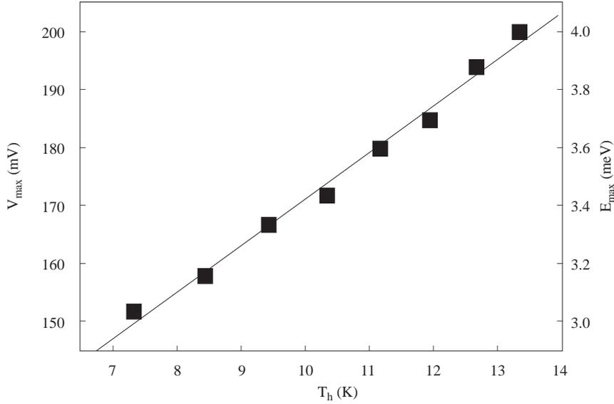
**Figure 4.** The position of the maximum,  $V_{max}$ , in  $\Delta I(V)$  as a function of heater temperature  $T_h$ . The right hand scale shows the corresponding phonon energy  $E_{max} = eV_{max}/n$ . The line shows a linear fit  $E_{max} = ak_B T_h + eV_0/n$  with  $a = 1.9$  and  $V_0 = 90\text{mV}$ .
