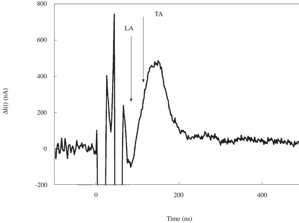
**Figure 2.** Time dependence of the phonon-induced signal  $\Delta I(t)$  for  $V=200\text{mV}$ ,  $B=0\text{T}$  and  $T_h=13.35\text{ K}$ . The vertical arrows show the expected arrival time of LA and TA phonons.
