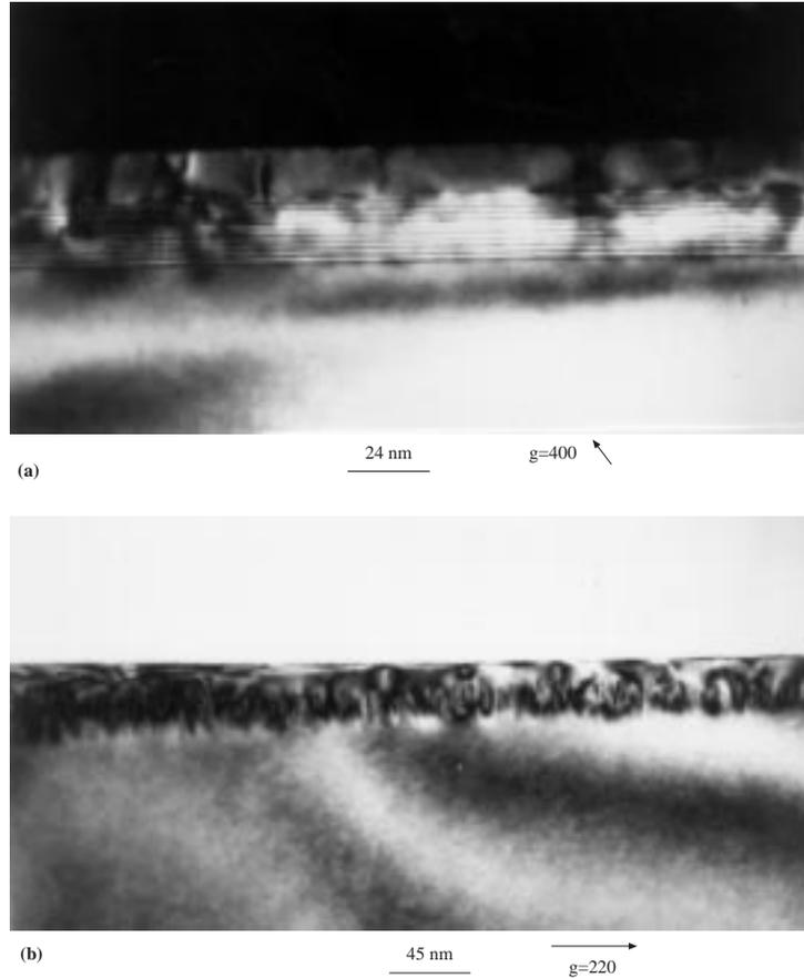
**Figure 1.** Dark-field and bright-field images of cross-sectional NU1537, (a) the sample is edge on, showing 10 InAs dotted layers in  $g=400$ , (b) misfit dislocations in  $g=220$ .
