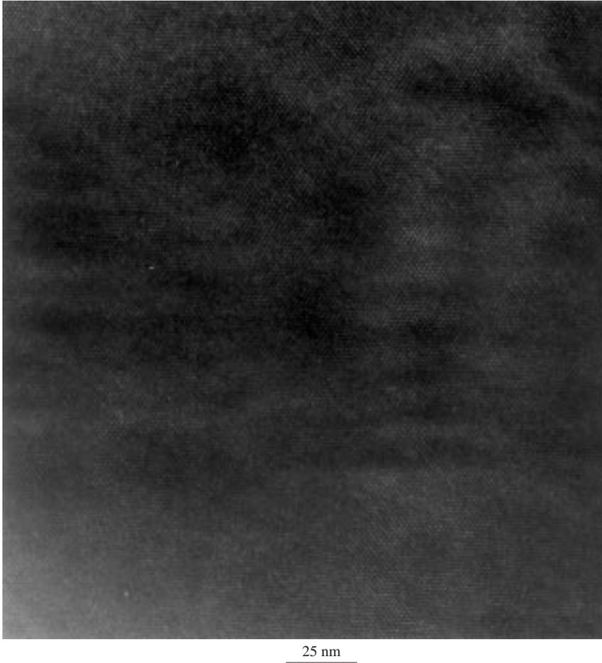
**Figure 2.** HREM image of NU1537 demonstrating the InAs layers with contrast in the  $[110]$  zone axis.
