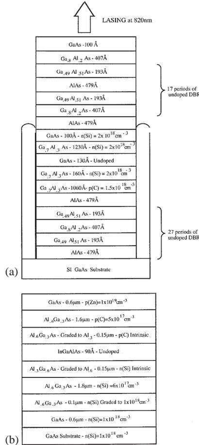
Figure 1. A schematic diagram of a) HELLISH-VCSEL and b) GRIN SCH QW laser
