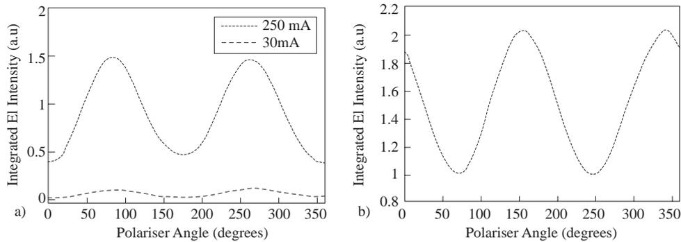
**Figure 6.** A comparison of light output polarisation for a) edge emitting QW laser above and below threshold current and b) HELLISH-VCSEL with  $1\text{KVcm}^{-1}$  at 300K.
