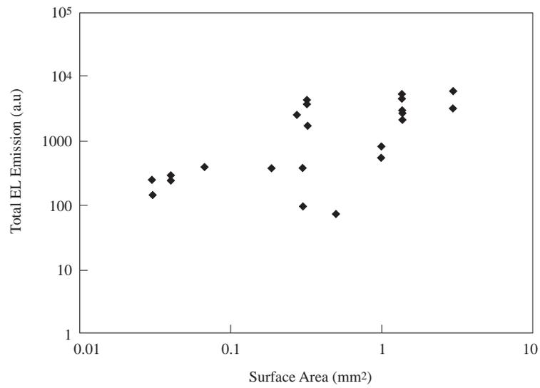
**Figure 7** Total EL intensity as a function of device surface area at 300K for HELLISH-VCSEL.
