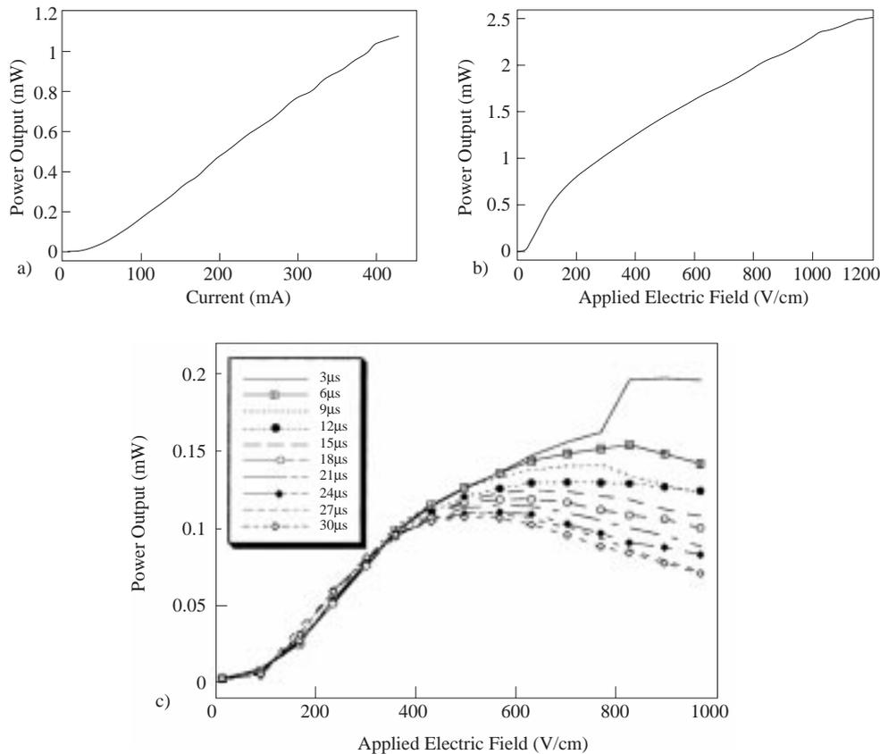
**Figure 5.** Output power of a) 1mmx30  $\mu\text{m}$  QW laser using pulsed power supplies, b) 3x1mm HELLSH-VCSEL bar and c) HELLSH-VCSEL output power as a function of applied voltage pulse width, with a constant repetition rate of 10ms at 300K.
