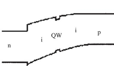
**Figure 3.** The simulation of the original p-i-n device.
