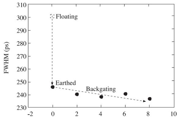
**Figure 9.** FWHM of the response as a function of back gating voltage
