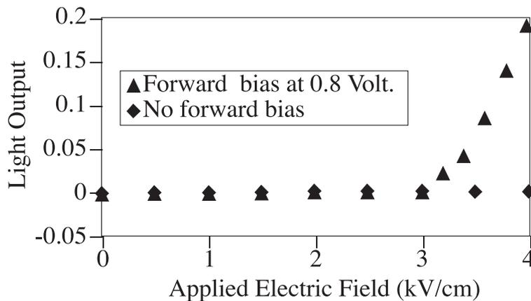
**Figure 5.** Light output as a function of the applied electric field
