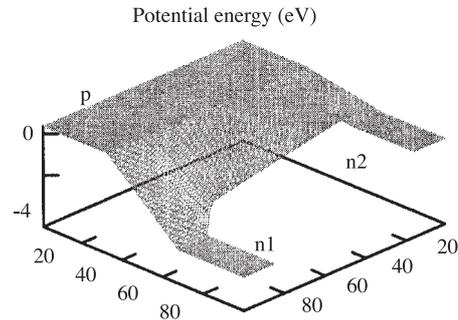
**Figure 8.** The potential energy profile with 5V applied across the two top contacts.
