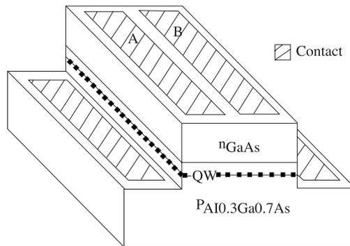
**Figure 2.** A The test device
